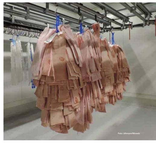
A loop label is printed out at goods receipt for each weighing unit - in this case, bacon pages on the hook -, attached and managed as a goods receipt batch.
