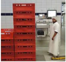
The pallet is weighed at the disassembly exit and is given a barcode label.
